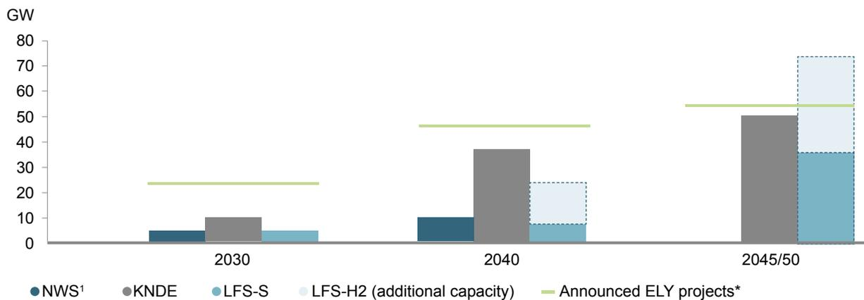
Projections shown: NWS: National Hydrogen Strategy, KNDE: Klimaneutrales Deutschland 2045, LFS: Langfristszenarien (-S: electricity scenario, -H2: hydrogen scenario). Areas with dashed outlines show theoretically needed electrolysis (ELY) capacity assuming an electrolysis efficiency of 70% and 3,500 full load hours.
