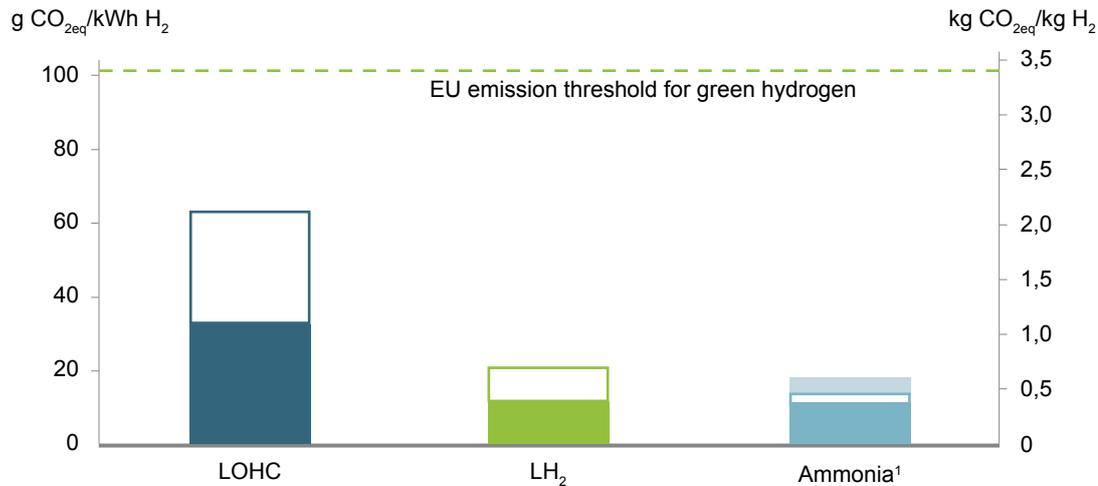
White area: additional emissions from shipping LOHC-carrier molecules or metal tanks back to the port of origin.
