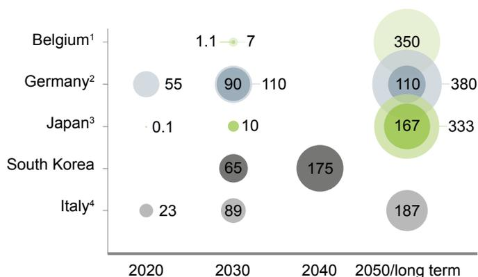
Bubble size and corresponding labels show the targeted lower (inside bubble) and upper (outside bubble) range of annual demand for hydrogen and derivatives in TWh per year.
