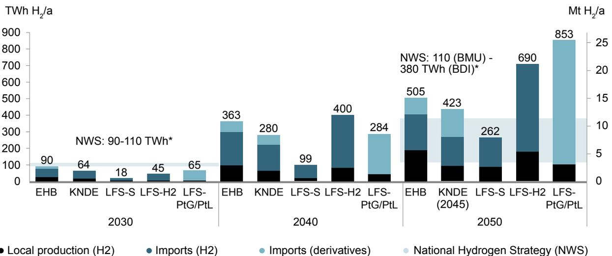
Projections: NWS: National Hydrogen Strategy, EHB: European Hydrogen Backbone, KNDE: Climate-Neutral Germany 2045, LFS: Langfristszenarien (-S: electricity scenario, -H2: hydrogen scenario, -PtG/PtL: power-to-liquid/power-to-gas scenario). \* Includes both hydrogen and PtG/PtL demand.
